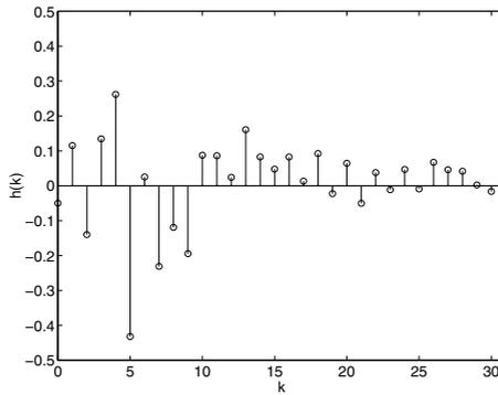
**Fig. 2.** A 32 tap non-minimum phase convolutive channel
