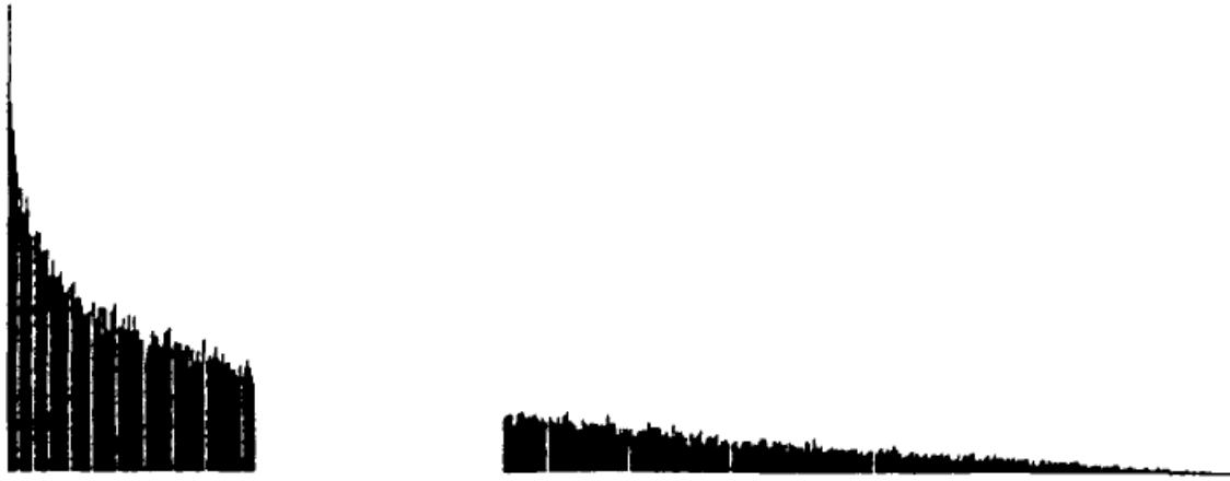
Figure 8. Probability density function showing regions of equal area.
