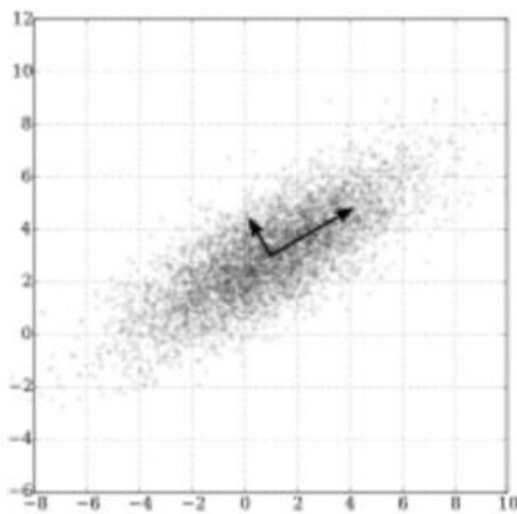
PCA of a multivariate Gaussian distribution centered at (1,3) with a standard deviation of 3 in roughly the (0.866, 0.5) direction and of 1 in the orthogonal direction. The vectors shown are the eigenvectors of the covariance matrix scaled by the square root of the corresponding eigenvalue, and shifted so their tails are at the mean.
